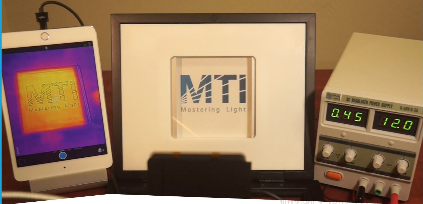
Above: Glass covered with NanoWeb® is placed over the MTI logo where 12 volts are applied. On the left, the tablet shows the heat signature of the glass measured with an infrared camera. The glass reaches a temperature of 45 degrees Celsius within the first minute.
