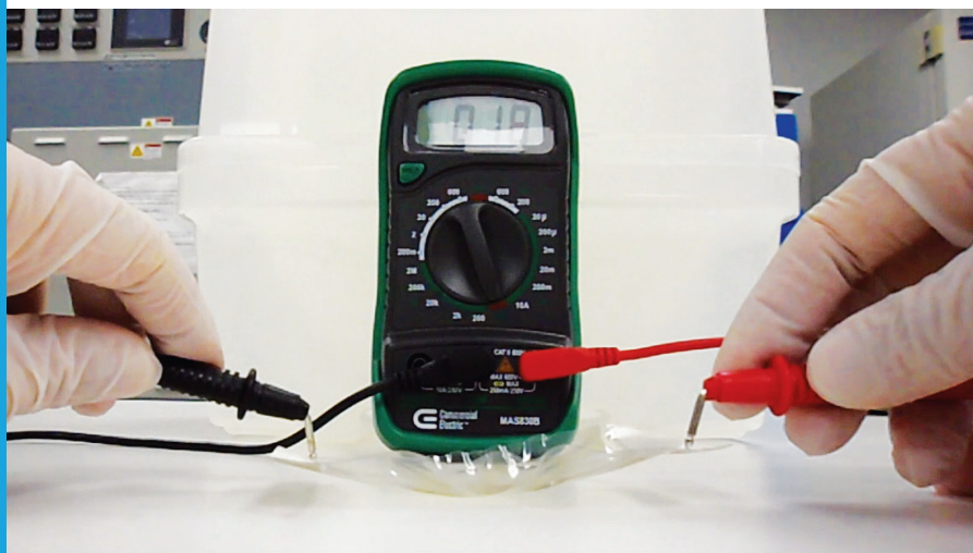
Above: Nanoweb®'s electrical properties do not change after it has completed the thermoforming process.
